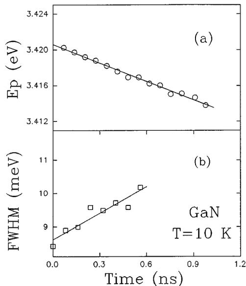
FIG. 3. (a) The peak positions  $E_p$  and (b) the full width at half-maximum (FWHM) of the 3.42 eV emission line as functions of delay time measured at  $T=10$  K. The solid lines are the least-squares fits using  $E_p(t) = E_p(0) - \alpha t$  and  $\text{FWHM}(T) = \text{FWHM}(0) + \beta t$ .
