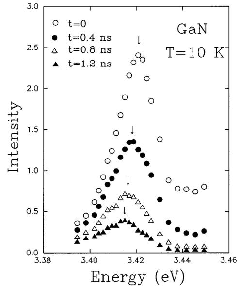
FIG. 2. Time-resolved photoluminescence spectra of the 3.42 eV emission line measured at  $T=10$  K. The arrows indicate the spectral peak positions at different delay times. Delay time  $t=0$  has been chosen at the positions of the maximum intensity in the luminescence temporal responses as shown in the inset of Fig. 1.
