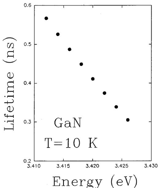
FIG. 4. Emission energy dependence of the recombination lifetime of the 3.42 eV emission line measured at  $T=10$  K.
